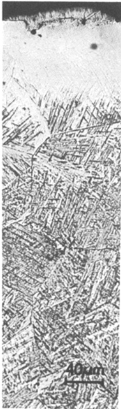
Figure 10 Ti electrode treated in Ar; etching TMi 37Ti.
