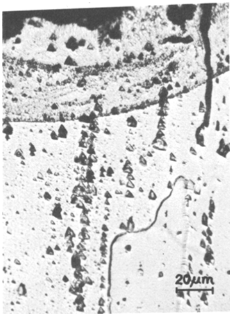
Figure 8 Plastic deformation in duralumin; etching T46HF + 46H 2 O + 8HCl.
